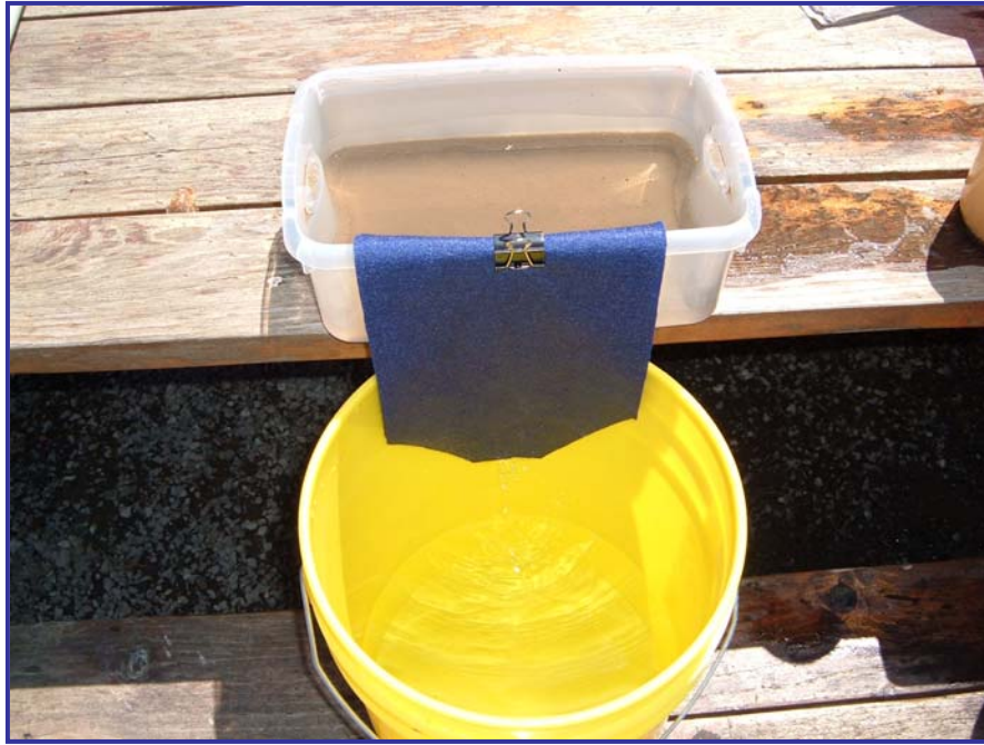
Figure 8 Capillary filtration of turbid water
